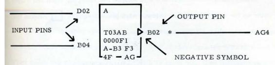
Notice that the input and output pins will be shown at the point where a signal enters or leaves the block.
